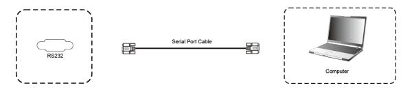
After using serial port cable to connect central control equipment and machine, certain function of the machine can be controlled via central control equipment, such as: machine ON/OFF, and adjustment of sound volume, etc.
